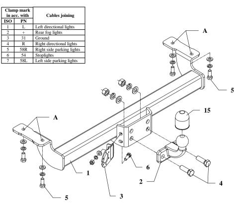
This towing hitch is designed to assembly in following cars: **SUZUKI VITARA, 5 doors,** produced since 1995, catalogue no. **W05** and is prepared to tow trailers max total weight **1875 kg** and max vertical load **75 kg**.
