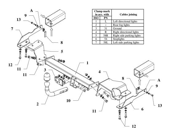
This towbar is designed to assembly in following cars: **Toyota Yaris CP10** (**Japanese version**), produced since 1999 till 2001 and **Toyota Yaris CP10** (**French version**), produced since 2002 till 2005, catalogue no. **O24** and is prepared to tow trailers max total weight **900 kg** and max vertical load **50 kg**.
