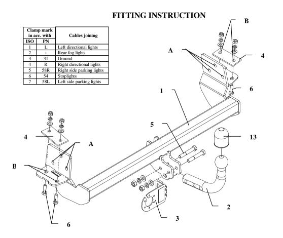
This towbar is designed to assembly in following cars: **TOYOTA COROLLA ESTATE E11** produced since 07.1997 till 07.2001, catalogue no. **O17** and is prepared to tow trailers max total weight **1400 kg** and max vertical load **75 kg**.
