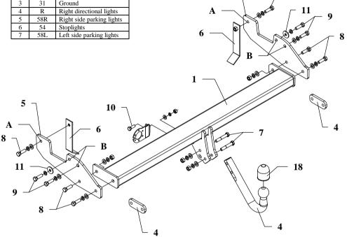
This towbar is designed to assembly in following cars: TOYOTA HILUX 4x4 with double cabin, produced since 2005, catalogue number O64 and is prepared to tow trailers max total weight up to 2500 kg and max vertical mass 100 kg.
